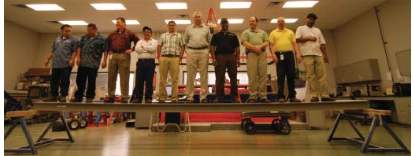
XL6 strength demonstration: Under a uniform load of 30 psf, deflection on a 20' span is L/180.
